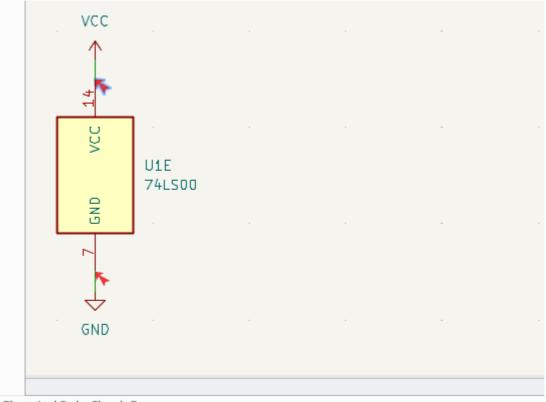
Electrical Rule Check Error Input Power pin not driven by any Output Power pins To avoid this warning, connect the net to PWR\_FLAG symbol on such a power net as shown in the following example. The PWR\_FLAG symbol is found in the power symbol library. Alternatively, connect any power output pin to the net; PWR\_FLAG is simply a symbol with a single power output pin.
